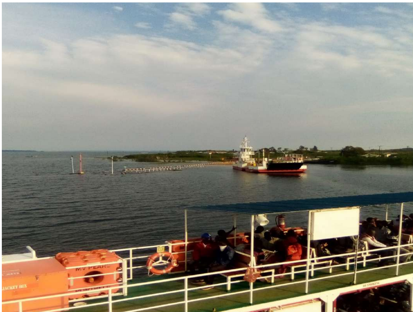
A typical scene at Bukakatta Landing. In the foreground: MV Pearl sailing to Luku Landing; In the background-Grounded Ferry- MV Ssesse, Submerged jetty, gum pole fenders totally underwater, navigation lights and gangway banisters partly seen
