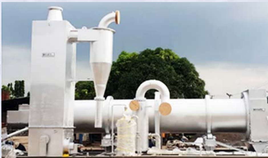
Boskel High Temperature Rotary Kiln Incinerator for destruction of hazardous industrial and medical wastes
