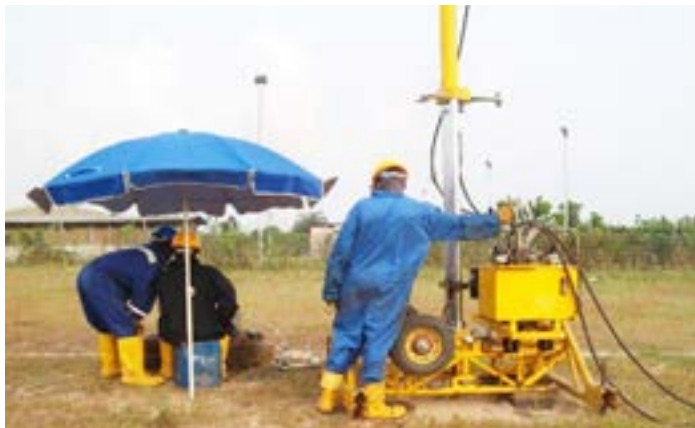
A cone penetration test site
