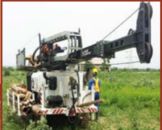
LX6 Multipurpose Rotary Rig with Capacity to drill up to 600m
